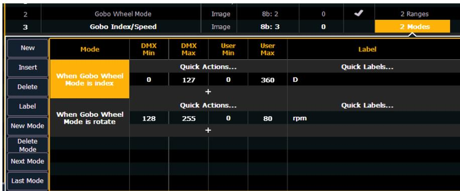
Assign the DMX and user values. The range values were used for the DMX values. For index, the user values were set to 0-360 degrees. The quick label for degree unit was used so the degree symbol will display in the encoder display. For rotate, the user values were to 0-80 rpms.
