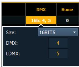
You can alter the default DMX address assigned to any parameter in the list. This is not the actual address that will be used when patched, but rather it is the order of address for the parameter relative to the other parameters in the fixture.
