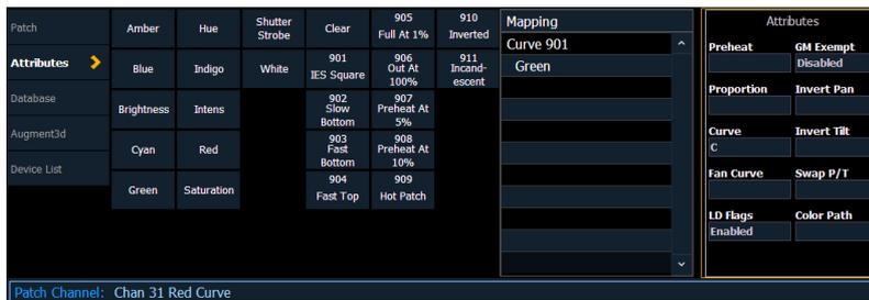
Eos provides ten pre-programmed, commonly used curves. They can be edited or copied to a new curve location. When a pre-established curve is deleted, it will return to its original state.
