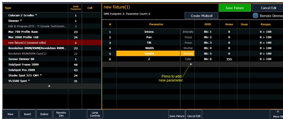
3. Determine the total number of parameters that your fixture has. Do not count 16-bit parameters as two parameters, this will be done in a later step.
