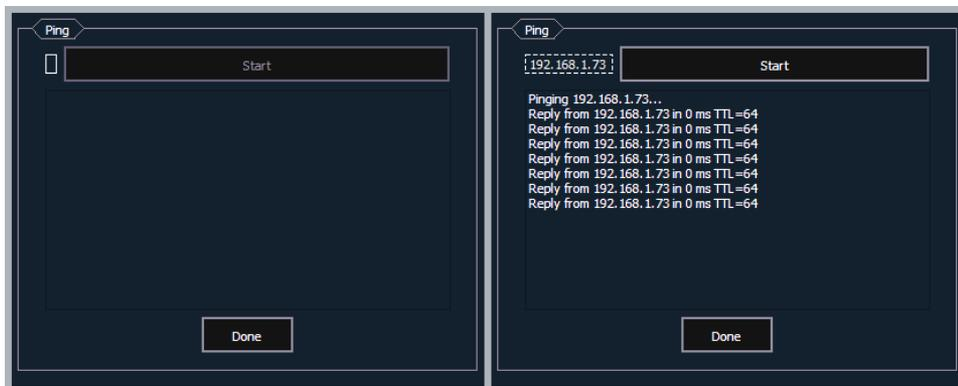
1. Click the empty box on the left, and enter the IP address of the device you want to ping.
