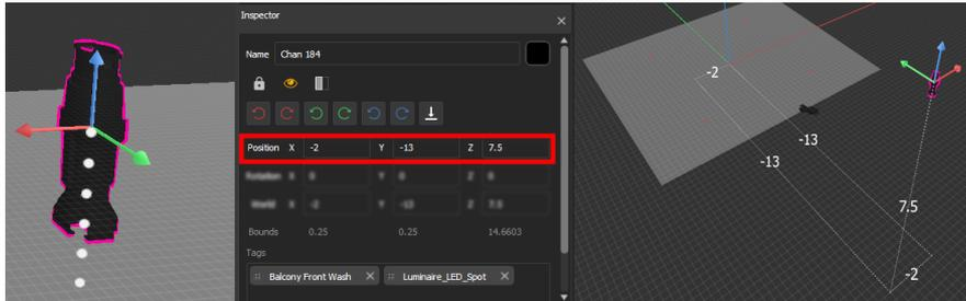
In the above example, the fixture patched to Channel 184 is -2 meters offset on the X axis, -13 meters offset on the Y axis, and 7.5 meters offset on the Z axis.
