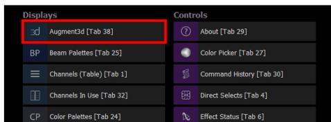
Either open a new tab and select **{Augment3d}** from the Displays list, or hold down **[Tab]** and type **[38]**.
