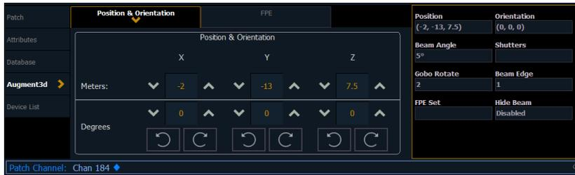
Under the Augment3d section in Patch, fixtures have fields for XYZ Position and Orientation. If the fixture is nested, this data is relative to the parent. World Position and Orientation are absolute, relative to the scene overall. If nested, an arrow indicator will appear next to the position and orientation fields. For more information about nesting, see [Nesting Objects](#).
