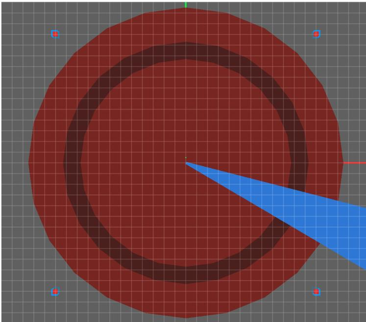
There are many ways to select FPE Point positions. The preferred method is to use at least 4 points close to the bounds of your space, as in the example above. Larger angles between points reduces the possibility of redundant information being used in the calculation. It may help to think of the points as outlining the base of a 3D shape that should cover as much of your space as possible.
