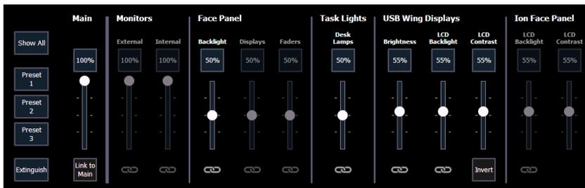
This menu allows you to adjust the brightness and contrast settings for your console's face panel, as well as any internal monitors, supported external monitors, fader wings, and task lights. All sliders have a range from 0% (dimmiest) to 100% (brightest).
