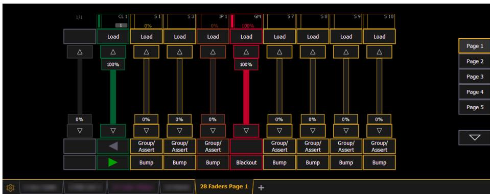
The virtual fader module has a configuration menu, which is accessed by first selecting the module tab and then double clicking on the tab to open the menu. With the virtual fader module selected, you can also select the gear icon, which is located by the tabs, to open the configuration menu.
