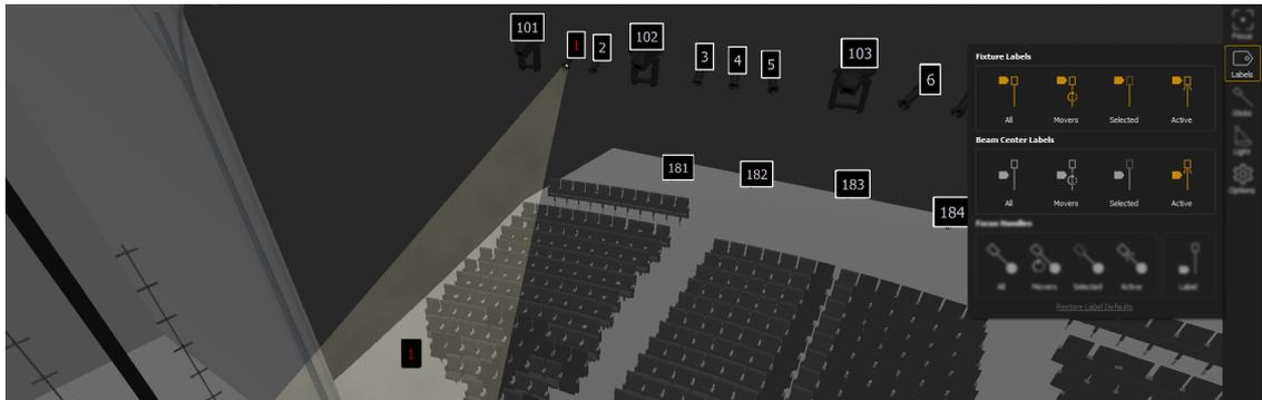
Fixture Labels display the channel number of the fixture. This can be useful in identifying which fixture is creating a particular beam of light.
