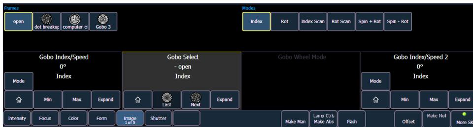
Directly under the middle two encoders are six hardkeys that are for encoder control. From left to right, these encoder paging keys control intensity, focus, color, shutter, image, and form. Pressing any of these will change the parameters controlled by the encoders.
