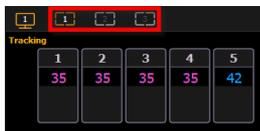
These three monitor icons are used to switch between each monitor's available workspaces. Each can be set up to include any of the desired layout, displays, and controls options offered on the [Home Screen](#). Double-clicking on any of the icons will jump all connected monitors to that workspace number.
