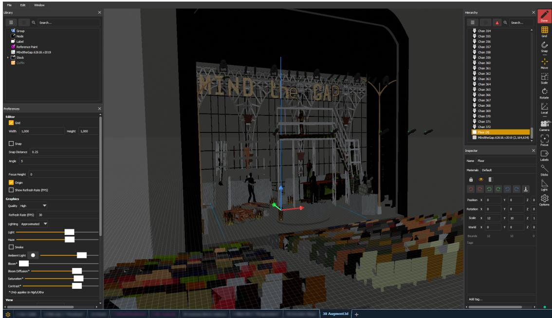
Surrounding the central workspace are primary windows to assist in fixture and object manipulation: the Library, Materials, Preferences, Hierarchy, and Inspector. These windows can be freely dragged, rearranged, re-sized, and closed.
