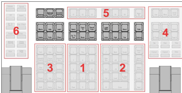
Backlit hardkeys are provided on the face panel. The brightness level for those keys can be adjusted in the [Brightness Settings \(on page 182\)](#).
