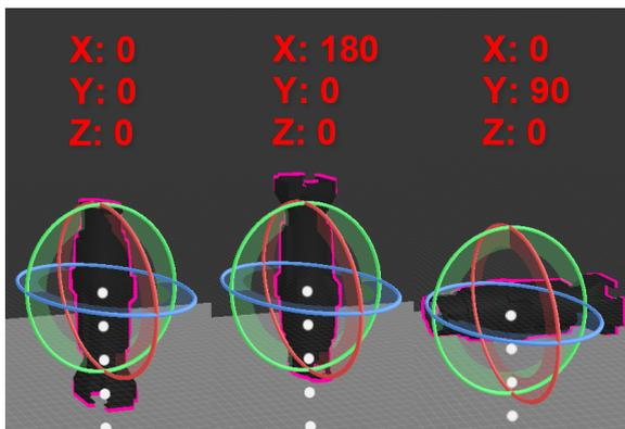
The above left example shows the default orientation of 0/0/0, or pointing straight down. The center shows a rotation of 180° about the X axis, pointing the fixture straight up. The final example shows a rotation of 90° about the Y axis, pointing the fixture to the side.
