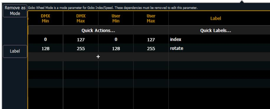
After patching the new fixture, you will be able to check your modes in the encoder display and ML controls. There are now buttons for the modes, and for index, the degree symbol is displayed with the user value.
