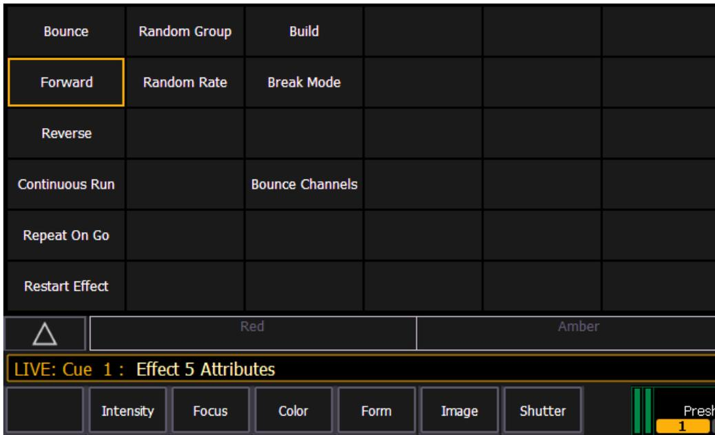
{Restart Effect} is an attribute that can only be accessed from this display. When enabled, {Restart Effect} will cause an effect to restart whenever the cue is fired. This attribute is applied to the cue that the effect is stored in and not in the effect itself.
