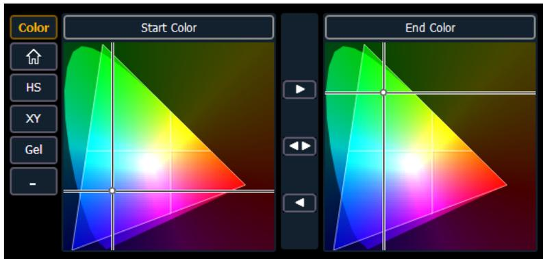
Using the buttons located between the two color pickers, you can also copy the start color to the end color, swap the start color and the end color, or copy the end color to the start color.
