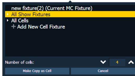
3. Select a fixture, a cell profile from an existing multicell fixture, or create a new cell profile by selecting **+ Add New Cell Profile**.
