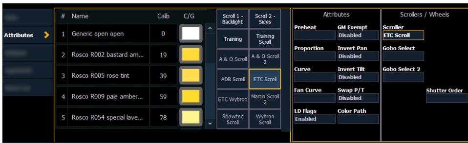
The picker displays on the left half of the CIA when you select the specific attribute (**{Scroller}**, **{Color Wheel}**, **{Gobo Wheel}**, or **{Effect Wheels}**). The picker displayed is specific to the selected attribute (the scroll picker will display when **{Scroller}** is pressed, the color wheel picker will display when **{Color Wheel}** is pressed, and so on).
