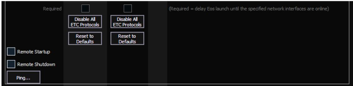
Using this button will disable all currently-enabled output, interface, DHCP, and SNMP protocols for the selected network port.
