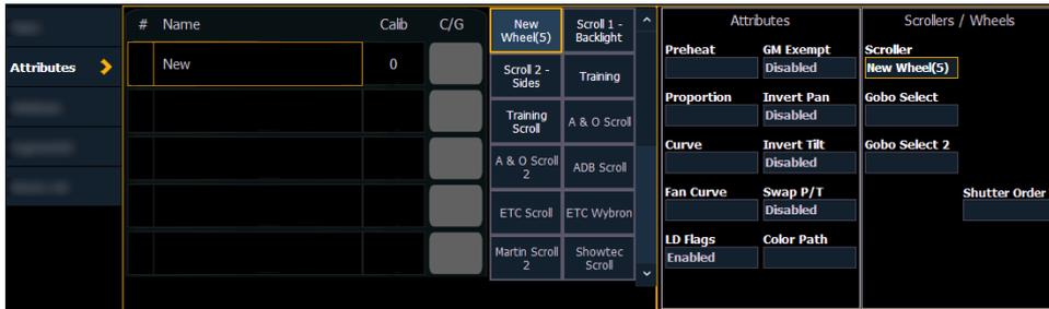
You can label the new wheel by pressing **[Label]** and typing the desired label on the virtual keyboard and pressing **{Enter}**.
