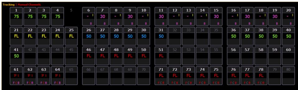
When the summary view has been collapsed to show only intensity data, you may include focus, color, or beam data in the summary view by holding down the **[Params]** key and pressing any parameter category key. This displays all categories again. On Element 2, you will need to use **[Data]**.
