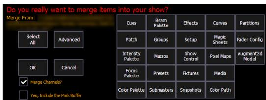
When Merge Channels is selected, channels from cues, submasters, groups, and other channel targets will be added to any existing channel targets of that same type.
