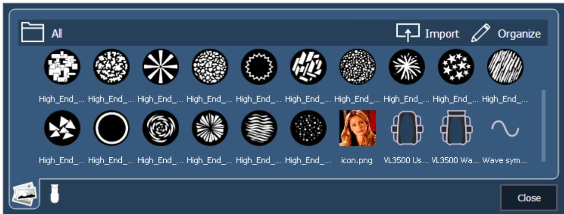
Any targets that can be applied to a direct select (other than channels and scenes) can be assigned an icon, which can be configured to appear on the direct select button in Direct Selects (Tab 4) or Custom Direct Selects (Tab 39). See [Custom Direct Selects \(on page 91\)](#) and [Configuring Direct Selects \(on page 89\)](#).
