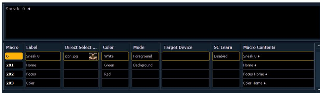
While in the macro editor display, any numeric entry on the command line is assumed to be a macro number. If the macro number entered already exists and **[Enter]** is pressed, the macro list will page to the selected macro and the macro content detail section will display all of the contents of the selected macro. If the macro number entered does not exist in the list and **[Enter]** is pressed, an empty macro will be created with the specified macro number.
