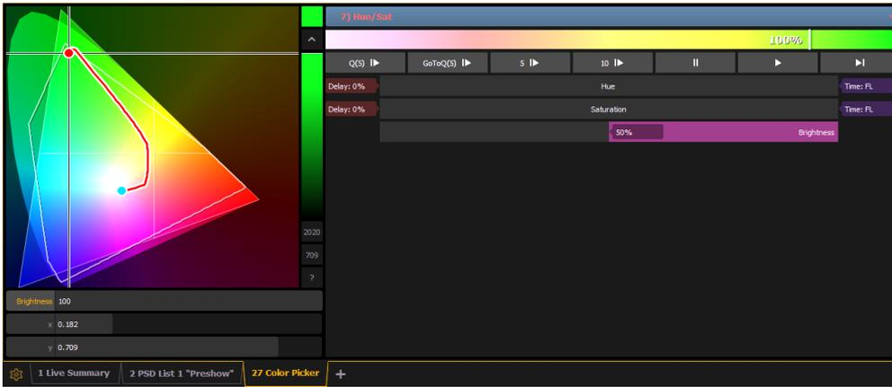
Changes can be stored in the destination cue as absolute data by using **[Update]** or **[Record]**. When there's a change to the color path information, a red c will display next to the channel number and the color path's name will display in red in the color path display. When that data has been saved, a blue c will display. The color path's name will also display in blue in the color path display.
