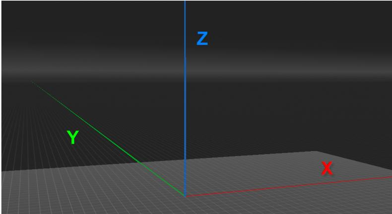
The point at the intersection of these axes (0,0,0) is the origin. This virtual point in Augment3d must correspond to a real point in your space, ideally on the floor. This could be in the center of your stage, in a corner, or any convenient point.
