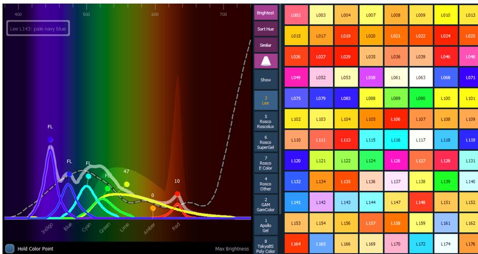
{Hold Color Point} allows you to adjust individual emitters and the other emitters will automatically adjust to hold the color selected. This can only be used with fixtures that have more than three color parameters.
