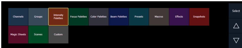
To open the direct selects, use the direct selects icon on the [Workspace Layout Menu \(on page 65\)](#) or [Tab] [4]. Direct selects for specific targets can then be opened using the corresponding button.
