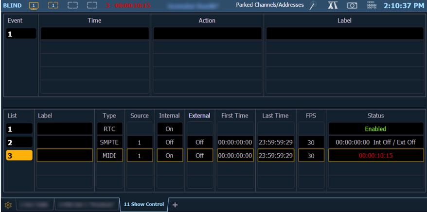
The screenshot shows the console interface with a top status bar displaying 'BLIND 1', '3 00:00:10:15', 'Parked Channels/Addresses', and '2:10:37 PM'. Below this are two tables. The first table has columns for Event, Time, Action, and Label. The second table has columns for List, Label, Type, Source, Internal, External, First Time, Last Time, FPS, and Status. The 'Status' column for List 3 is highlighted in red and shows '00:00:10:15'.
