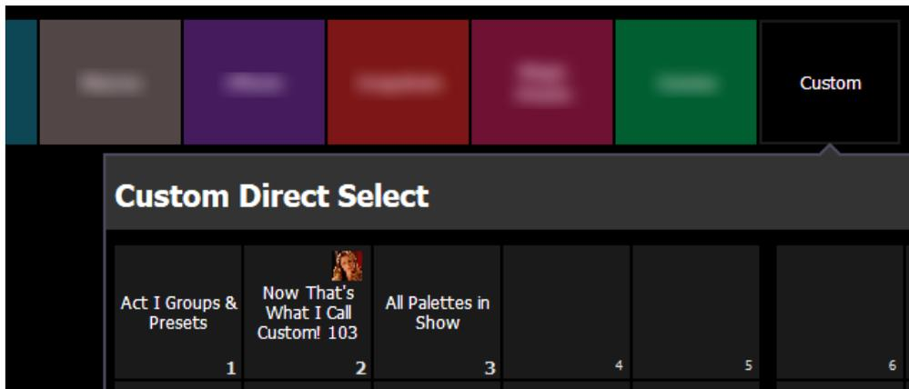
Once a custom direct select list is open, selecting an empty button will display a popup of the [Target Selection Menu \(2\) \(on page 91\)](#), allowing you to quickly assign a target or range of targets.
