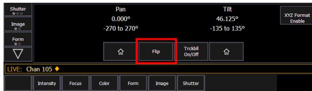
2. Test with pan values of -90°, 0°, and +90°. The fixture should point to the left, straight forwards, and to the right, respectively. If so, pan is mapped correctly. If not, follow the steps below to correct the pan range in the Fixture Profile Editor.
