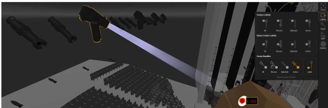
Focus Handles create a controllable point at the end of the beam of an automated fixture, which can be dragged to focus a single fixture, or multiple fixtures together while maintaining their spatial relationships.
