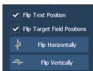
Allows you to flip objects horizontally or vertically. You have the option of also flipping the text position and / or the target field positions.
