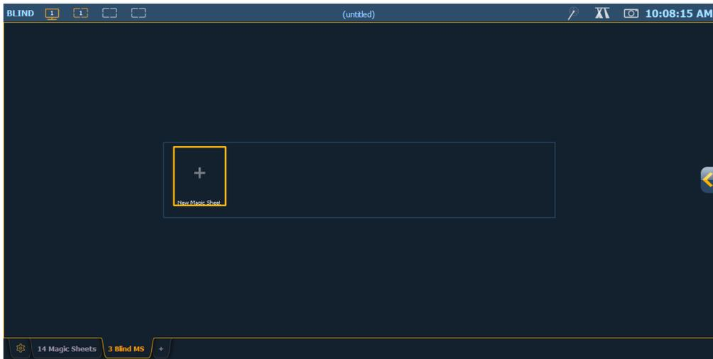
After you have created a magic sheet, you can recall a specific magic sheet, by pressing [Displays] {Magic Sheet} [#] [Enter] or you can navigate to **Displays> Record Targets> Magic Sheet** and press [Select] to open the magic sheet list (see [Magic Sheet List \(below\)](#)).
