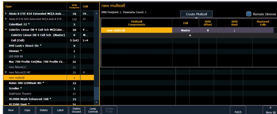
2. Press **{+}** to add cells. This will open a fixture list display. Only fixtures added to your fixture list will be here.
