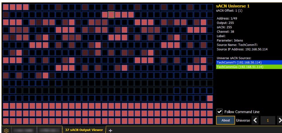
The left side of the viewer is the universe grid. It displays 512 address cells. Cells outlined in a color are currently patched addresses. Each patched cell contains an address number and output value. Unpatched cells are black and only have an address level.
