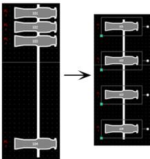
Set the distance you would like by placing the first and last objects. Then with all objects selected that you wish to distribute (including the first and last ones you positioned), click the **{Distribute Vertically}** button.
