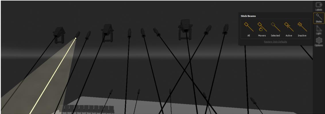
Stick Beams draws a line from the fixture to wherever the beam lands. Stick Beams do not require intensity and can be used to focus a fixture that is not currently outputting.
