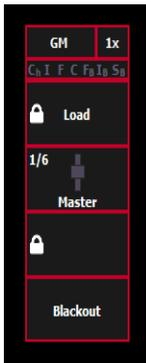
The first button is locked as a load button, and cannot be configured. The second button is disabled and cannot be configured. The third button can be configured as a blackout button or disabled. When configured as a blackout, both buttons must be pressed to set the grandmaster to blackout.
