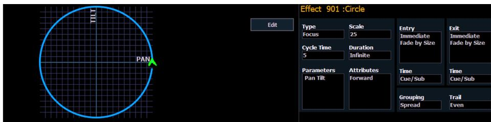
When adjusting the form of a focus effect, you can hold down **[Shift]** while using the horizontal encoder to change the vertical form.
