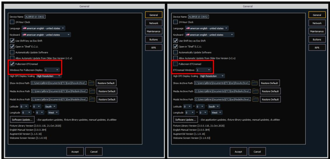
When the "Fullscreen ETCnomad" box is checked, ETCnomad will automatically launch fullscreen, on all connected monitors of your computer. Select "1" in the "Windows Per Fullscreen Display" dropdown to show a single fullscreen ETCnomad display on each monitor, or "2" to subdivide each fullscreen display into 2 ETCnomad windows.
