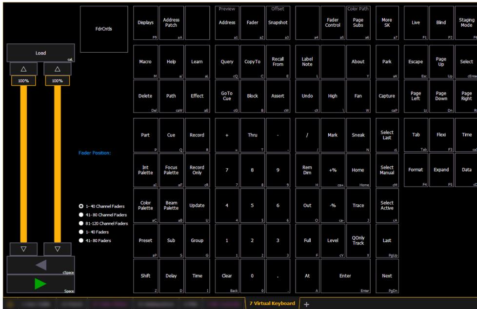
The virtual keyboard displays the alphanumeric keyboard shortcut for that hardkey in the lower right hard corner.
