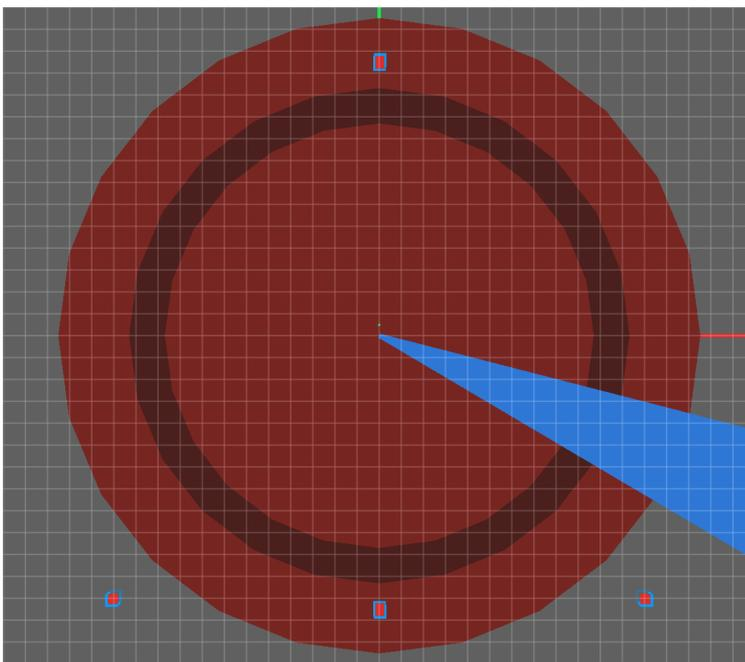
A better (but still problematic) configuration is pictured above. Since one of the points is in a line between two others, the data from that point is redundant and cannot be used to calculate the fixtures' positions.
