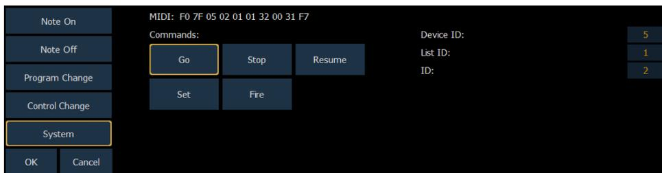
System commands allow you to specify specific MIDI Show Control messages that can be received and interpreted by the console. While any MIDI Show Control command that matches the configured Device ID will be executed normally, this type of event setup allows you to respond to messages sent to different device IDs, or take additional actions based on a show control command.
