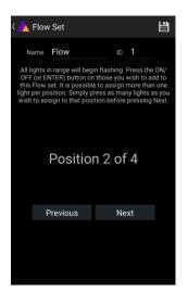
Now your lights will flicker every two seconds. To add a light to the currently shown positon of this set, press its button. Walk through the positions by "Previous" and "Next" and assign your lights. When finished, press the save button on top.
