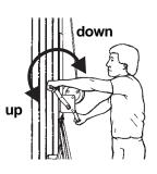
Result: The winch should operate smoothly, free of hesitation or binding.
