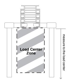
See the chart on the next page for maximum load centers for standard forks, adjustable forks and flat forks.
