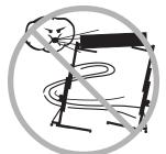
Do not leave a load raised when windy conditions may occur unless the machine(s) are properly guywired
