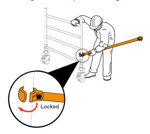
Position the second end frame as shown and fit the other end of the horizontal brace on to the vertical, just above the bottom rung. Fit a second horizontal brace on the bottom rungs on the other side of the frames to square the tower.
