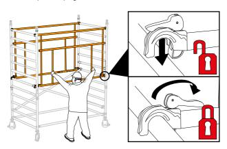
Fit the stabilisers (See notes on page 28). If required, fit a temporary deck on the lowest rungs of the tower. Fit a trapdoor deck on the 8th rung on one side of the tower. Ensure the trapdoor is positioned with the hinges towards the outside of the tower as shown. Fit a fixed deck next to the trapdoor deck on the 8th rung. The platform is now complete. Climb the end frame below the trapdoor on the inside of the tower.
