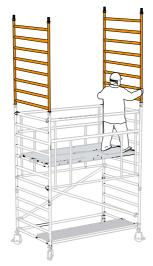
Fit two more AGRs to the end frames, with the top claws on the 20th rungs. Fit a trapdoor deck on the 16th rung, with the trapdoor in line with the one below. Place a fixed deck on the 16th rung next to the trapdoor deck.
