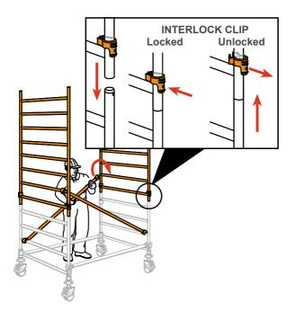
Fit an AGR on both sides of the tower. The bottom of the AGR must be fitted to the 6th rung of the tower, as shown. The AGR should be placed up against the end frame verticals.
