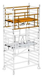
**9** Continue to add pairs of end frames, AGRs and fit decks as shown in the previous steps.
