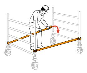
Fit two additional end frames and check the frame interlock clips are engaged. Fit two diagonal braces (blue) in opposing directions, from the 2nd rung to the 6th rung on the opposing side. Ensure the frames are vertical and level by checking with a spirit level and setting the adjustable legs as required.
